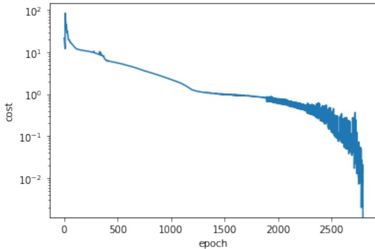
As we can observe from the above plot, the optimization was a bit of a bumpy ride towards the end. Situations like this can often be improved by decreasing the learning rate when approaching the minimum. For that we could have used one of the `torch.optim.lr_scheduler` classes or manually stop the optimization at some point, decrease the learning rate and resume from where we stopped.
